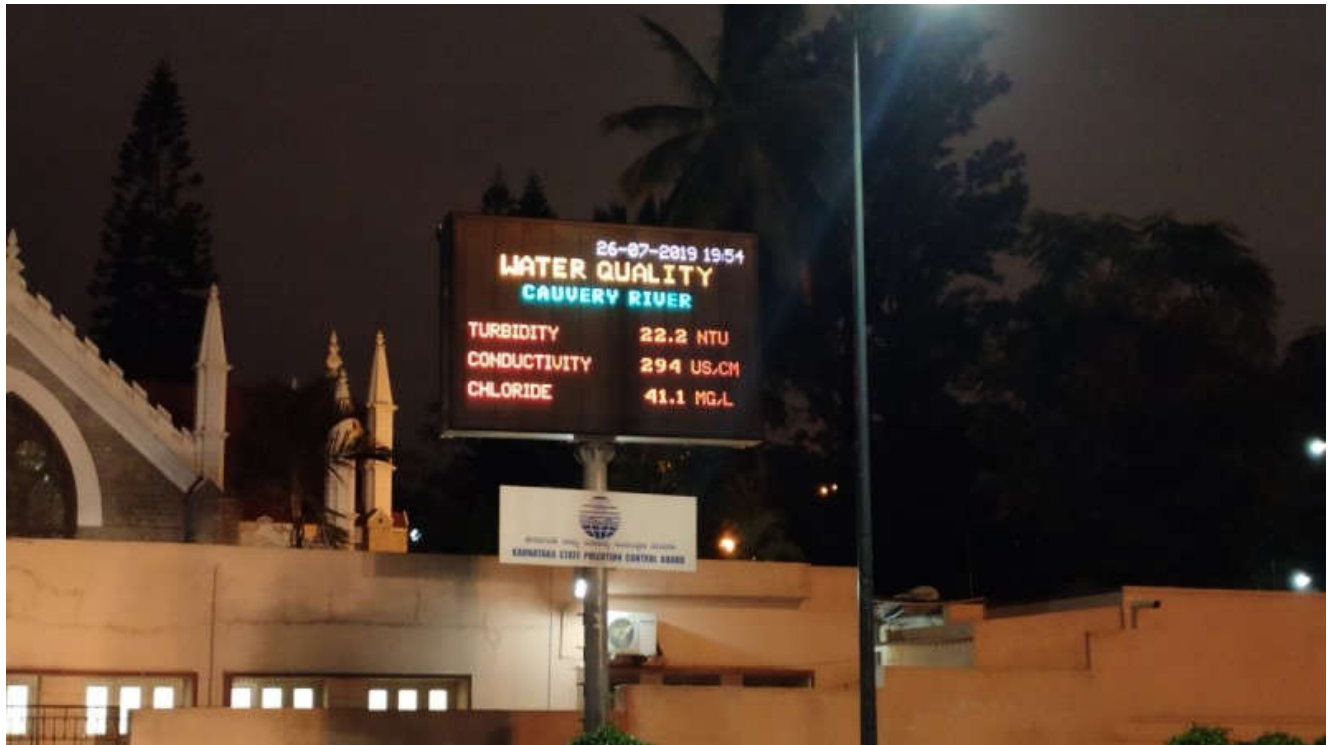
KSPCB monitor displaying water quality Amal Rasheedali
